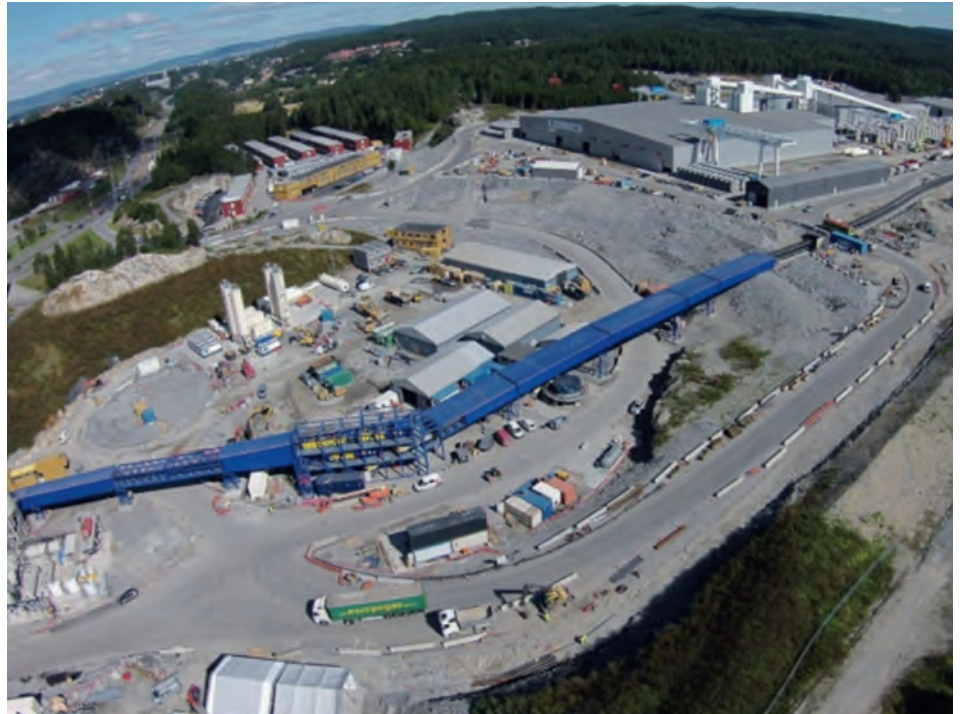
Figure 10 : Aerial view from the Åsland construction plant at the Follo Line Railway Tunnel showing conveyor belt, sorting plant and concrete lining segment factory.
