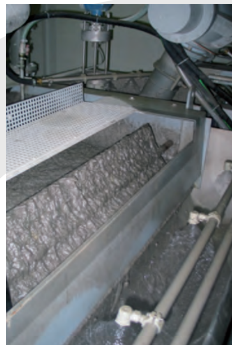
Figure 85 : Mica extraction by flotation technique (photo C. Thalmann)
