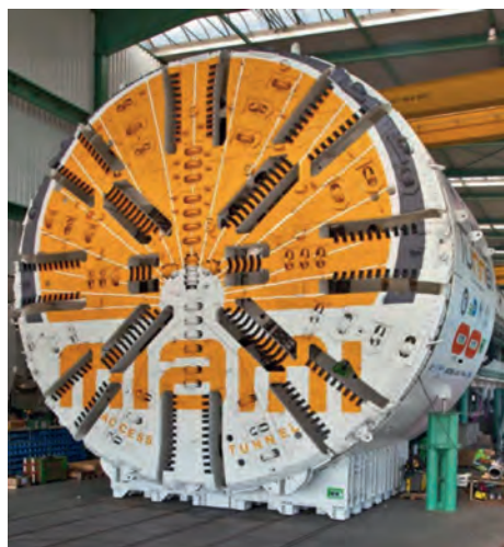
Figure 46 : One of the world's largest EPB machine (12.9m diameter) ready for the very challenging Port Miami Tunnel, in Miami, FL (photo from Herrenknecht).
