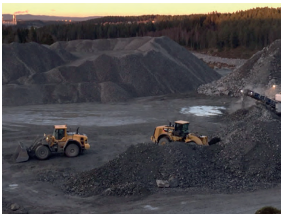
Picture 63 : Crushing and sieving plant for preparation of aggregates for different purposes. Follo Line Railway Tunnel Project, Norway.
