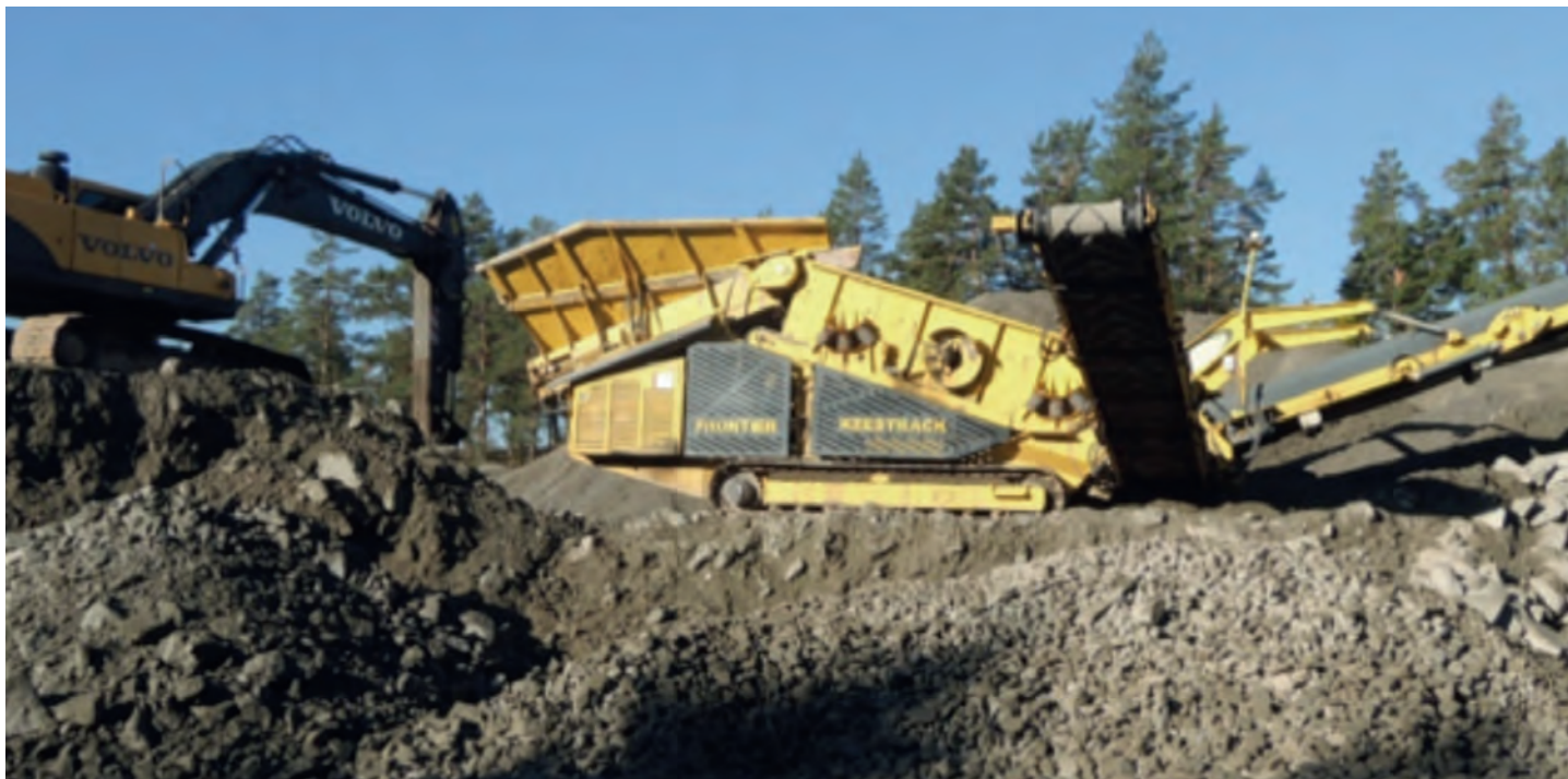
Figure 64 : Mobile crushing plant used for minor temporary works. Follo Line Railway Tunnel Project, Norway Bjørnar Gammelsæter 2015.
