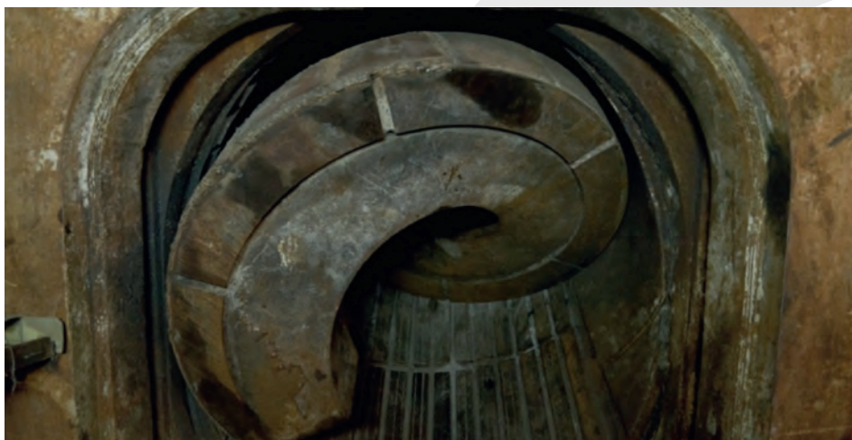
Figure 55 : Screw conveyor of "Bertha" at the SR 99 tunnel in Seattle, Washington USA.
