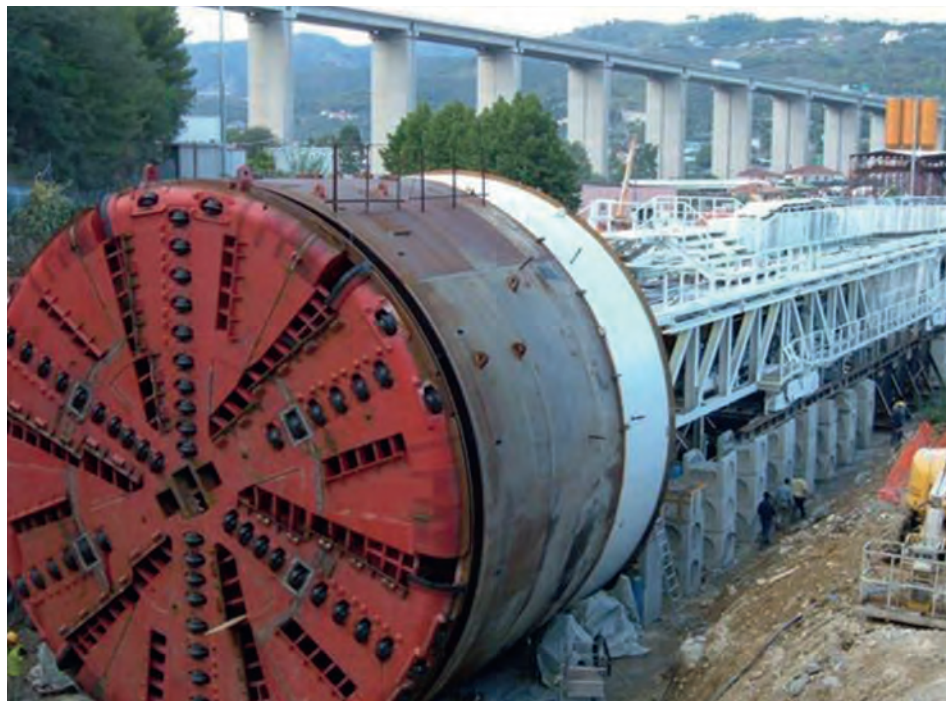
Figure 45 : EPB machine under mobilization at the C1 Andora – San Lorenzo Railway Link, Italy (Martelli Francesca, Italy).
