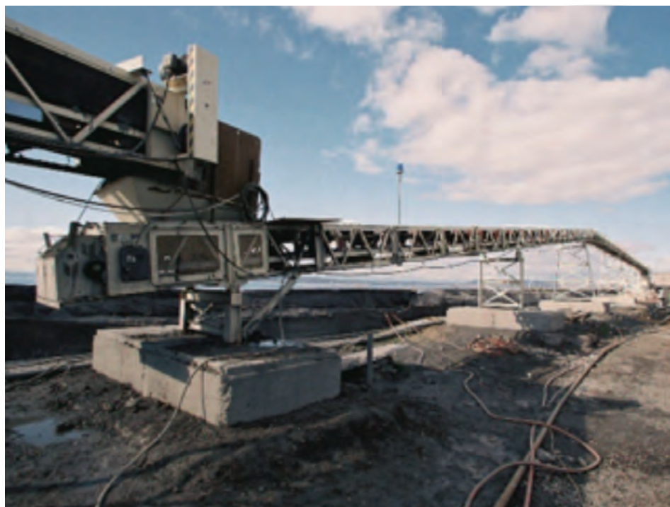
Figure 42: Brightwater Sewer Tunnel, Seattle, USA Tunnel muck (EPB TBM) on overland conveyors to marine loading and disposal site. (photo from B. Fulcher).
