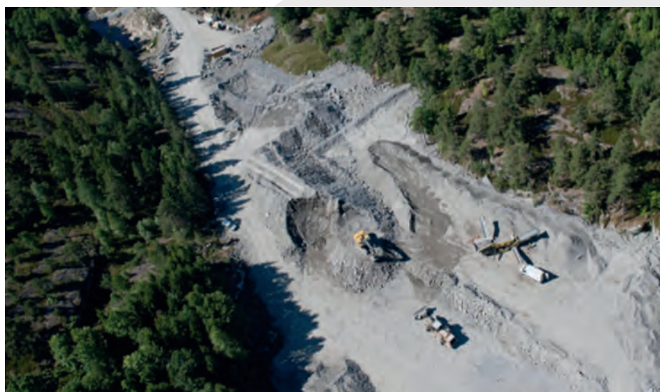
Figure 38 : Light processing plant for concrete production. Vestfoldbanen Railway Project, Norway, Lot 12.2 (Norwegian National Railway Authorities, NNRA).
