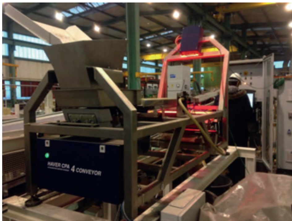
Figure 44 : Automated on-line grain size analysis (Reference 1).
