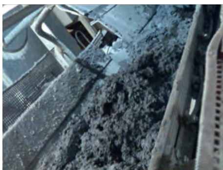
Figure 49 : Tunnel muck from EPB TBM machine, probably not useable for construction purposes, and must be considered as waste material
