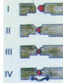
Stages for Seals Tightening Presstufen
