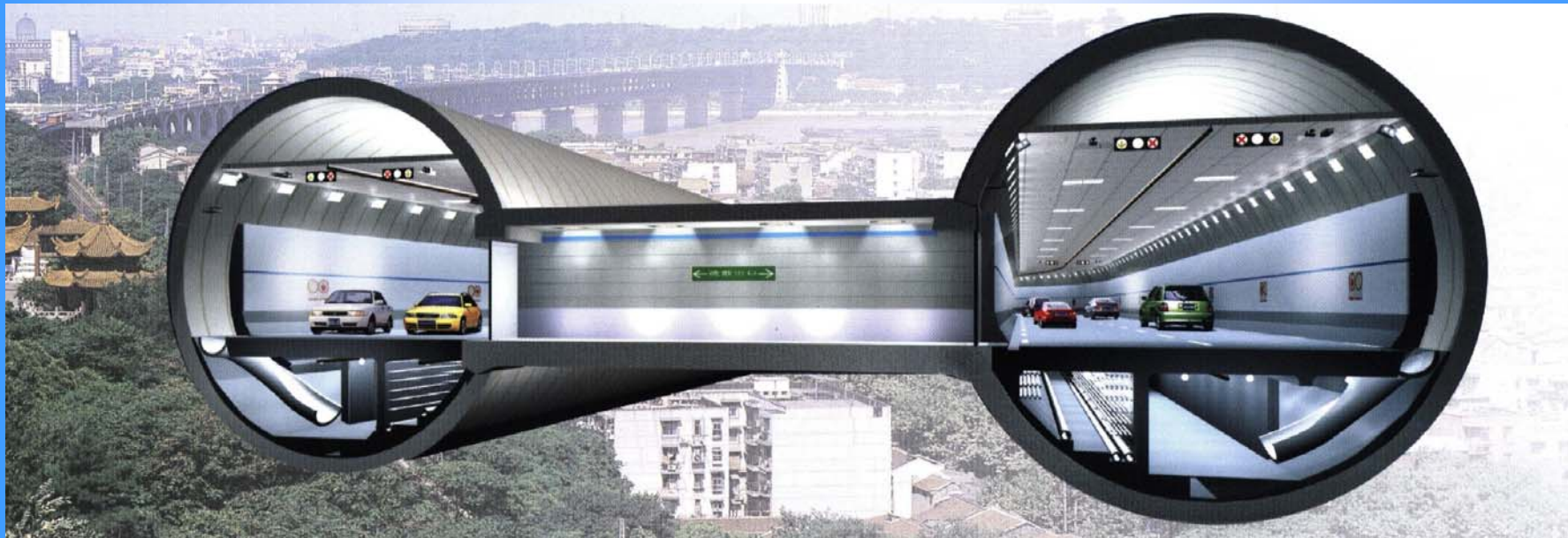
TBM Driven Unidirectional Tunnels with Cross Passages (Changjiang Tunnel Project, Wuhan)
