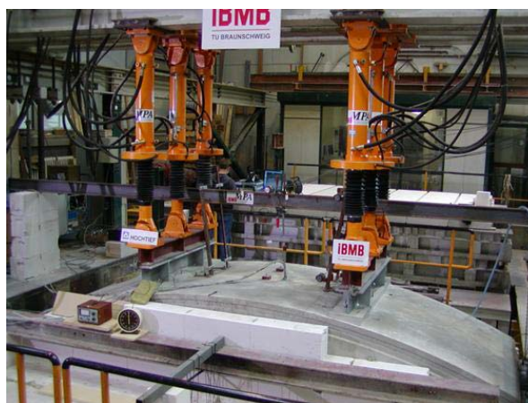
Fig. 6: Fire test with recently developed fire proof concrete at the TU Braunschweig, Germany under a fire load of 1200 °C over more than 90 minutes
