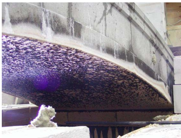
Fig. 7: Nearly no spalling effects after the test according to Fig. 6
