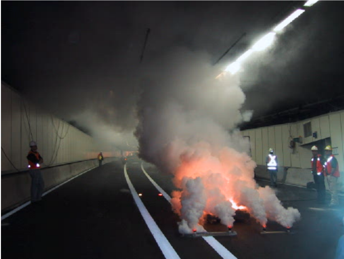
Figure 4 Hot Smoke Test M5 Motorway
