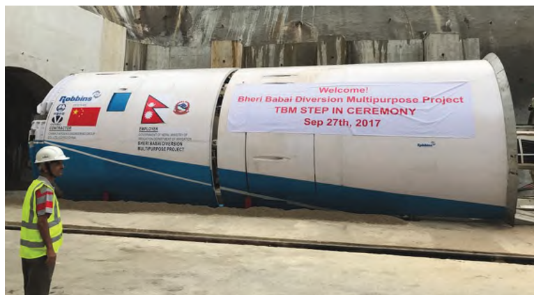
The 5.2m diameter Double shield TBM ready for excavation on the Bheri Babai Multipurpose Project
