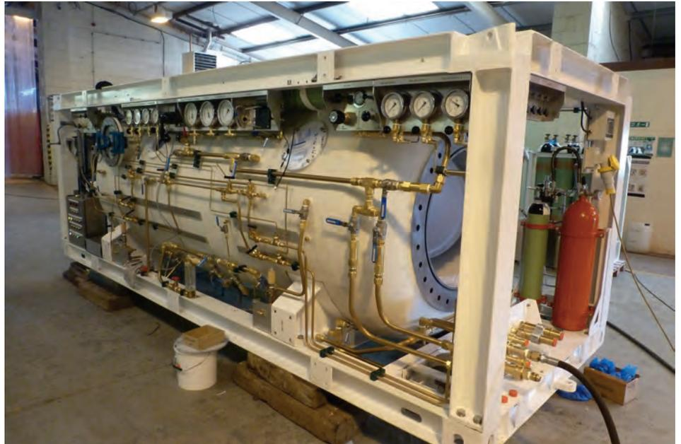
Figure 3 : TUP Shuttle at factory test
