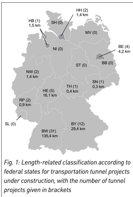
Fig. 1: Length-related classification according to federal states for transportation tunnel projects under construction, with the number of tunnel projects given in brackets
