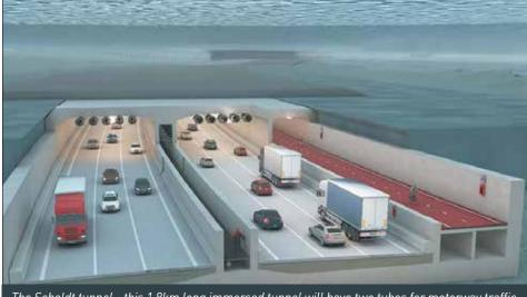
The Scheldt tunnel - this 1.8km long immersed tunnel will have two tubes for motorway traffic and a separate tube for cyclists and pedestrians.
