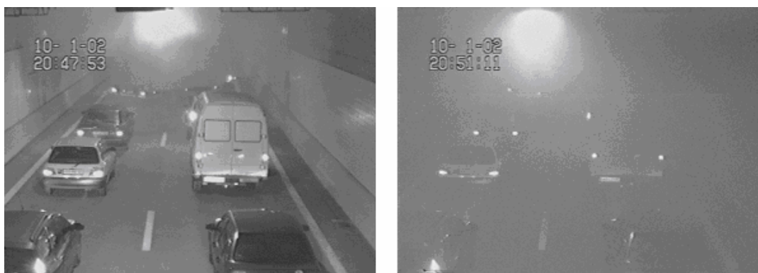
Figure 1 Cars at the front gradually disappear in smoke, but the drivers happily stay seated (field study, Boer 3, 4 ).
