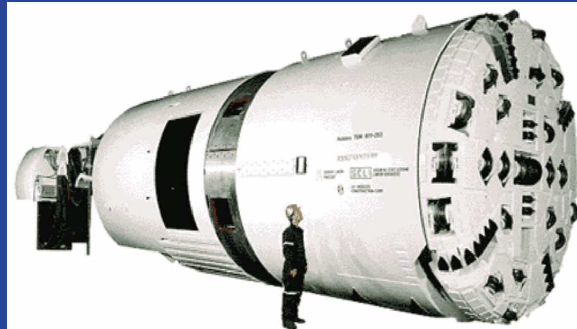
c) Double shield Robbins TBM
