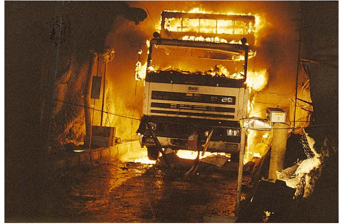
Fig. 9: Fire test with a heavy lorry within the scope of an European research project with substantial German participation (Brande in Verkehrstunneln, 1998)
