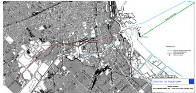
Plan view of Riachuelo River, the proposed sewer tunnels (red and green) and the emissary (also green)
