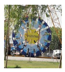
View of the Herrenknecht cutter head of an used shield machine, which presently is being refurbished by the Contractor, and of the typical tunnel profile
