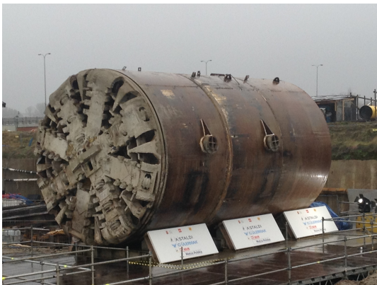
Fig 1. One of 4 TBMs EBP after execution of last tunnel section
