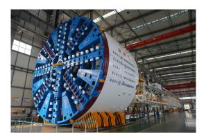
The Ø12.14 m EPB machine has been launched in Taixi railway tunnel project. This tunnel was mainly built in water rich aquifer layers sand, gravel, cobbles and clay.
