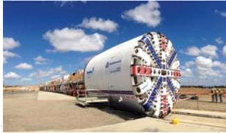
A Robbins TBM recently completed tunnel excavation for the Grosvenor Mine Access Drifts
