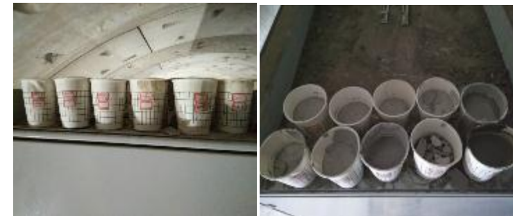
Synchronous grouting field sampling
