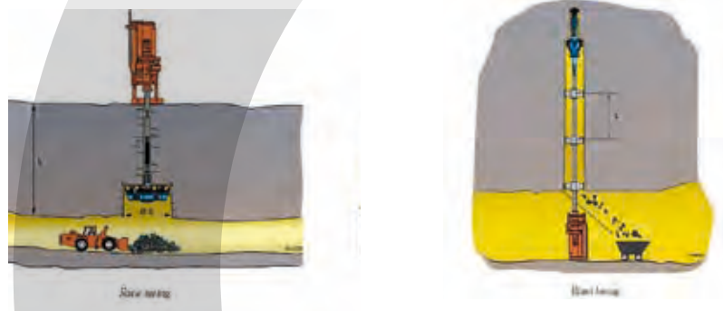
Figure 4 : Schematic drawing of Raise boring, horizontal boring, Raise drilling (or blind boring), Down reaming (Epiroc).
