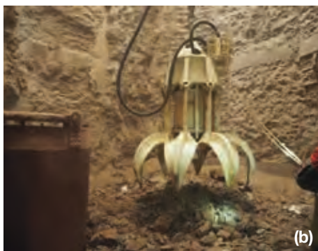
Figure 7 : (a) Clam shell Grab Bucket Shaft mucker (Slack, 2020), (b) Cactus Grab mucker (Niemann, 2020).
