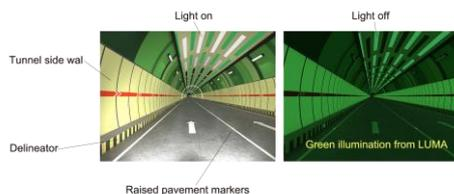
This project deals with a multifunctional energy-storage and luminescent material (LUMA) for sustainable and energy-saving lighting for tunnels. It is featured by energy storage, delayed luminescence, release of negative oxygen ions, dirt resistance, self-cleaning and antistaticity. LUMA has been applied in manufacturing a series of products including tunnel coating, tunnel
