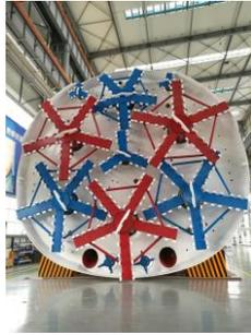
This project is a mechanized method with large section horseshoe shape EPB-TBM first applied in loess mountain tunnel. For mountain tunnel in loess, the conventional tunneling method is to use the sequential excavation method and double lining. The horseshoe shape multiple cutter heads EPB-TBM method have been made to replace the traditional one.
