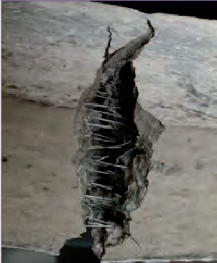
Steel Fibre Concrete after Breaking
