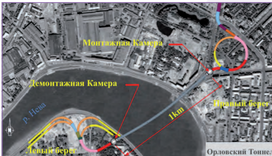
Plan View of the Orlovski Tunnel
