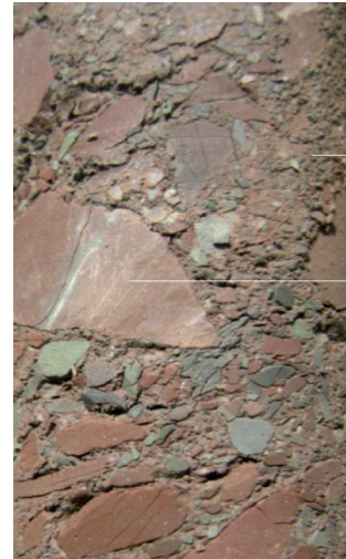
Figure 19 : Gibraltar tunnel. Breccia specimen consisting of a clay matrix with hard inclusions
