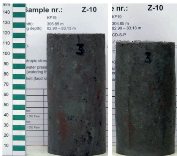
Figure 21 : Gibraltar tunnel. Breccia specimen before and after CD-testing [33]
