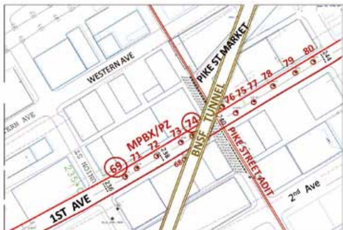
Figure 30 : TBM crossing at BNSF Tunnel and Pike Street Adit.
