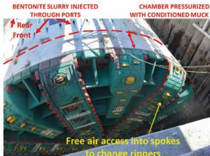
Figure 24 : EPBM cutter head in launch shaft, Alaskan Way Viaduct Replacement Tunnel.
