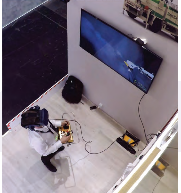
Figure 46: Normet concrete spraying simulator – Top: the “cave”, or Bottom: Virtual Reality Headset approach
