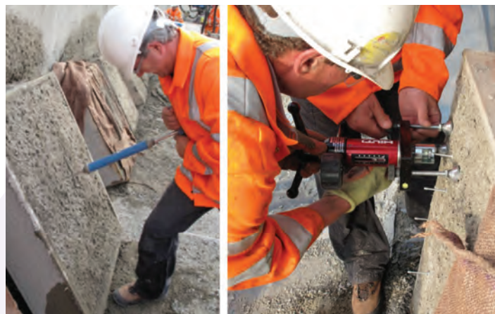
Figure 23: Current best practice for early age sprayed concrete strength measurement – Proctor penetration needle and Hilti pull-out method
