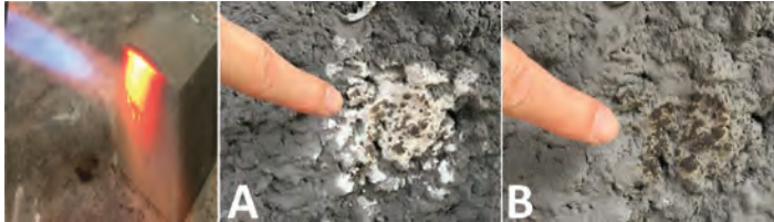
Figure 50: Effect of propane torch on a 4-5 hours old fly ash grout after 1 min fire exposure (1300°C)
