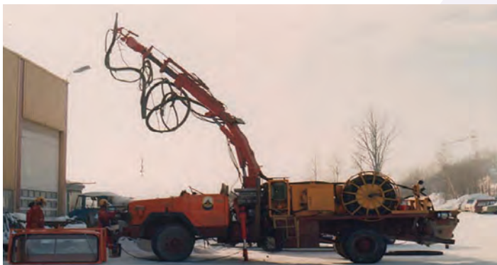
Figure 28: The Robocon "cabriolet", the spraying robot from eighties based on truck chassis (O. Woldmo/Robocon)
