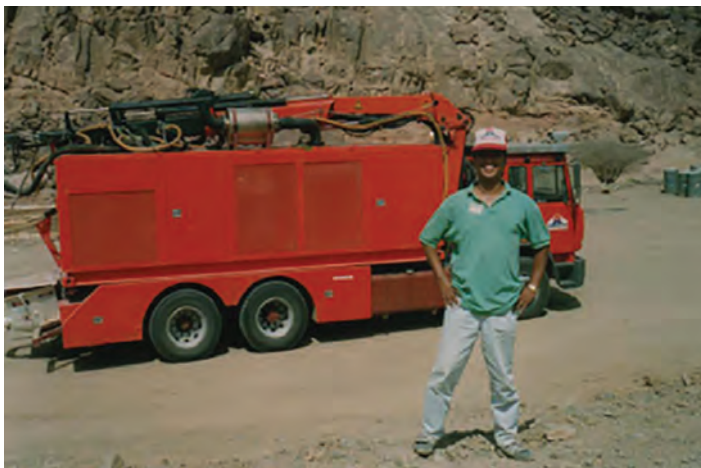
Figure 29: Truck based Robocon spraying robot from nineties with a video camera to record rock (O. Woldmo/Robocon)
