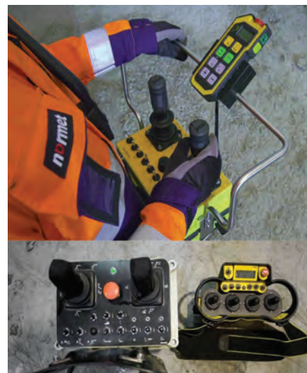
Figure 33: PIC Display –recording all of function of the spraying equipment and Pump
