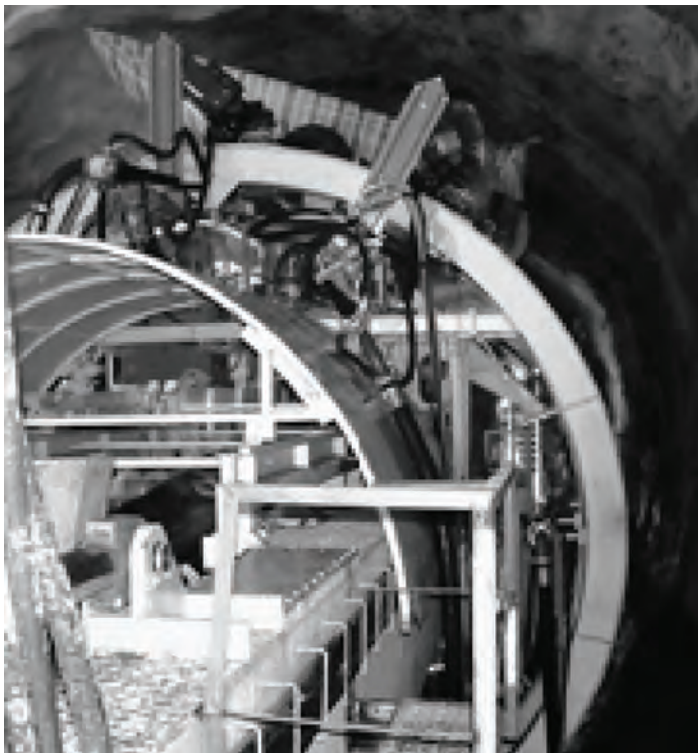
Figure 38: The MEYCO® Robojet spraying manipulator is integrated into a large diameter TBM (Source Meyco)
