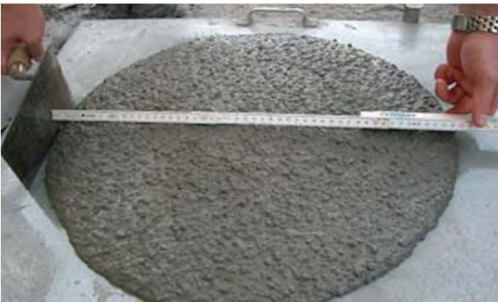
Figure 18: Flowable sprayed concrete mix has over 550 mm flow measured on a flow table (Melbye 2006)
