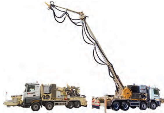
Figure 34: Normet Spraymec NorRunner 140 DVC is the biggest mobile sprayer in the world
