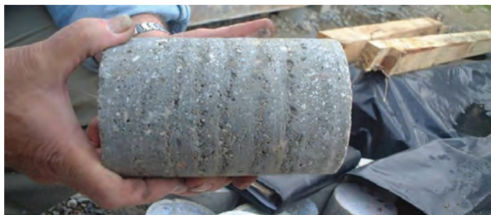
Figure 40: Pulsation will result in layering effect in the applied sprayed concrete
