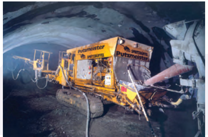
Figure 30: Putzmeister Buffalo spraying robot with two separate robotic spraying booms and concrete pumps (Source Putzmeister)
