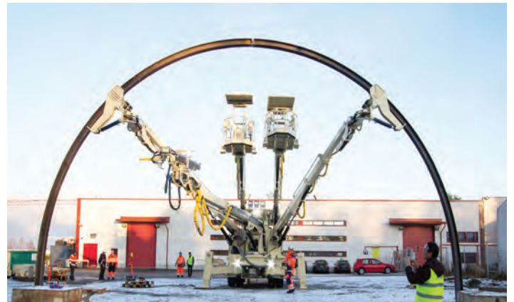
Figure 35: Normet Zeus-5 boom sprayer, working platform and arch-lifter in tests at the Normet factory before delivery to Japan
