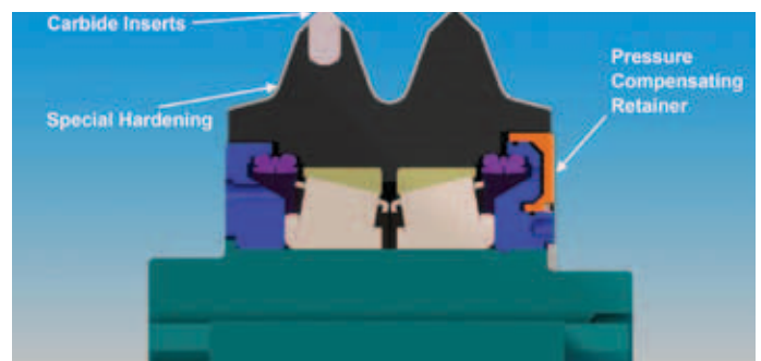
Figure 15. Pressure Compensated Carbide Insert Cutter
