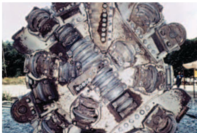
Figure 5. Test TBM for water jet-assisted cutters
