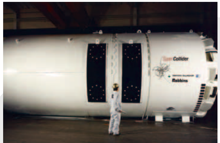
Figure 8. Side View of the Triple Shield Tunneling Machine
