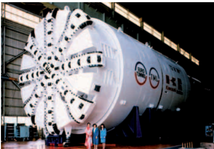
Figure 11. Channel Tunnel Hybrid articulated shield machine, French Side
