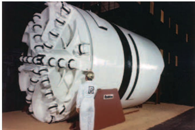
Figure 4. The first Double Shield Tunneling Machine, for Italy's Orichella project
