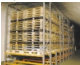
Figure 7 Commodity set-up for test 1 (wood pallets and plastic pallets).
