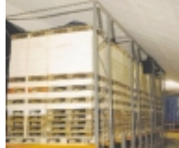
Figure 8 Commodity set-up for test 2 (wood pallets and PUR mattresses).
