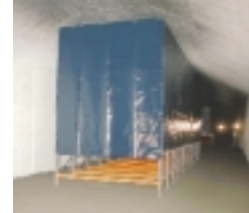
Figure 8 Commodity set-up for test 2 (wood pallets and PUR mattresses).
