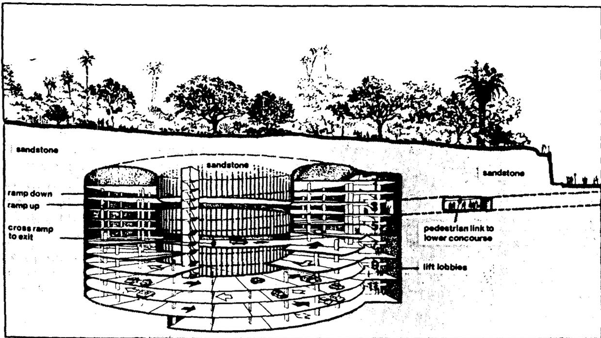
Figure 5. Architect's sketch of the double-helix Sydney Opera House Underground Car Park (Source: "Earthmover and civil contractor—Project report" [July 1992]).
