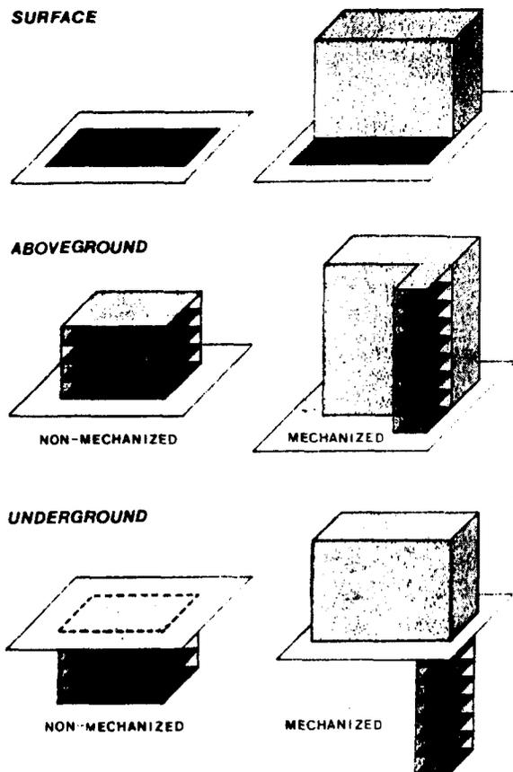
Figure 13. Structural types of parking facilities, categorized by location in relation to the surface.
