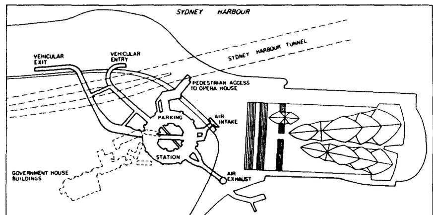
Figure 4. Location plan of the Sydney Opera House Underground Car Park (Source: Pells 1993).
