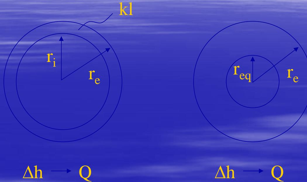
$$r_{eq} = r_e \left( \frac{r_e}{r_i} \right)^{-k_g/k_l}$$
