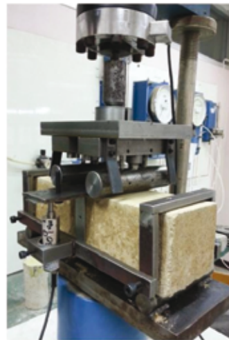
Figure 11: Four point bending test set-up
