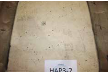
A specimen from fire testing (2 hour HC curve) with 1 kg/m³ polypropylene fibre.
