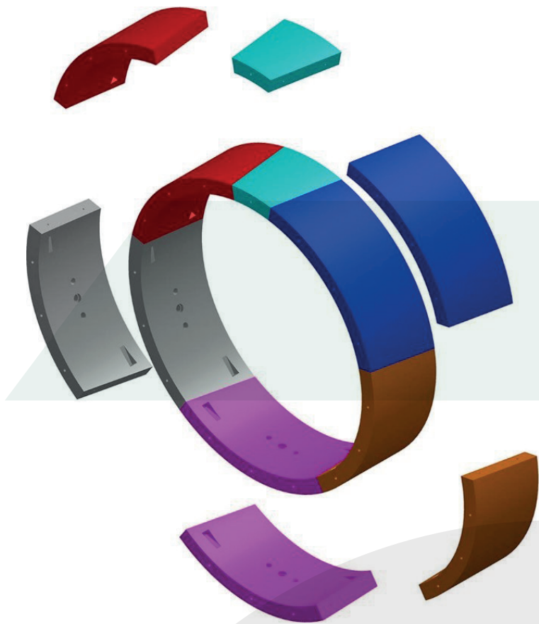
Figure 6: Ring Model as exerted from ITA-AITES Guideline for the Design of Segmental Tunnel Linings.
