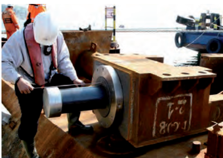
Figure 9 : Realignment jack
