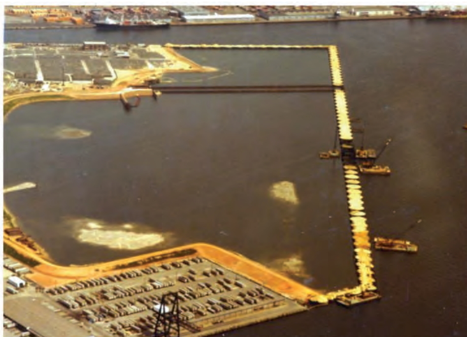
Figure 3 : Disposal site for hydraulic dredged material from tunnel trench. Note division between foreground area used for dredged sandy material, and the far area used for muck. (Future container terminal)
