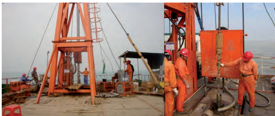
Figure 1 : Boring rig and SPT testing for the Hong Kong Zhuhai Macao immersed tunnel
