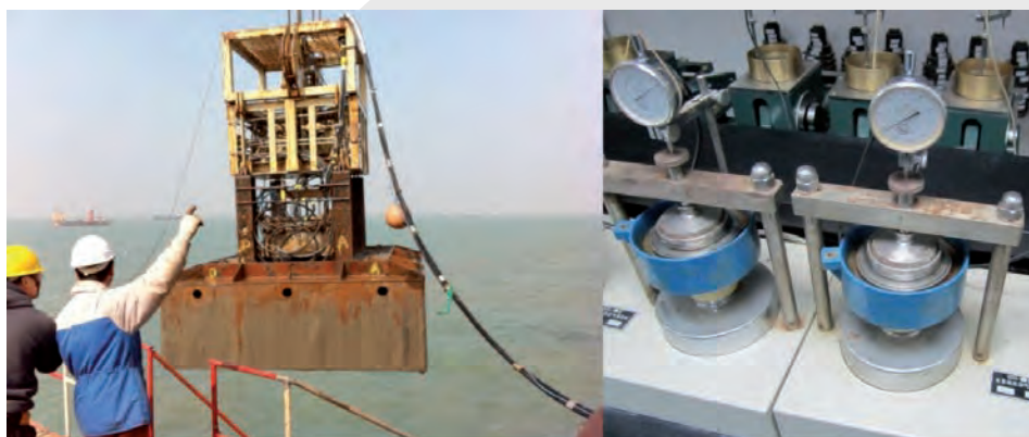
Figure 2 : CPTU equipment in use and Oedometer test cells for the Hong Kong Zhuhai Macao immersed tunnel
