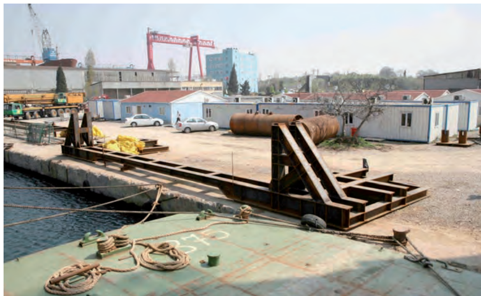
Figure 8 : Realignment Jacking frame
