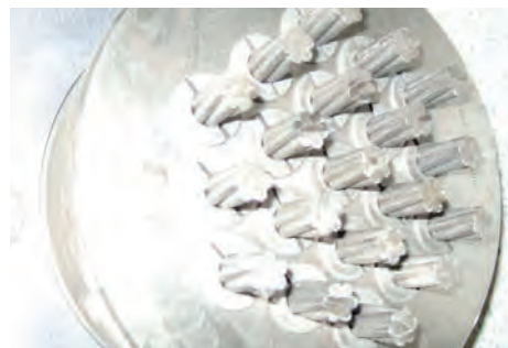
Figure 4 : 19 Strand cable and individual wires showing in anchor head (incl. wedges)
