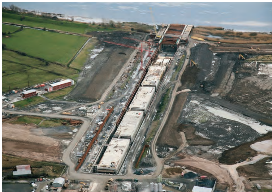
Figure 5 : Limerick tunnel elements in tunnel approach
