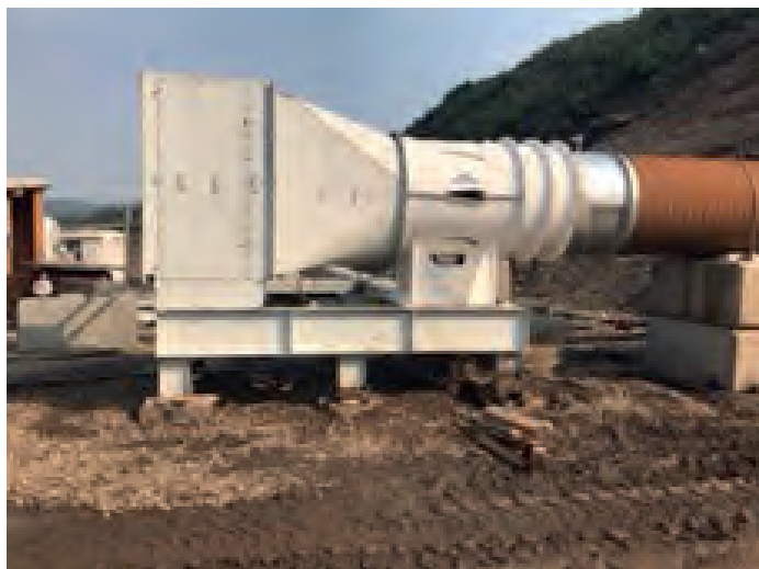
Figure 13: De-Duster – Fixed Mounted Demo Unit General arrangement of a De-Duster unit; linked to the tunnel ventilation system. (Courtesy Englo, Inc.)
