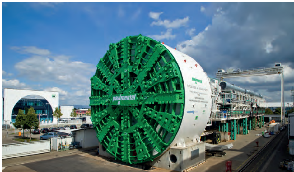
Figure 24: Santa Lucia Tunnel Boring Machine Fully assembled Earth Pressure Balanced TBM on-site for the Santa Lucia tunnel project in Italy.
