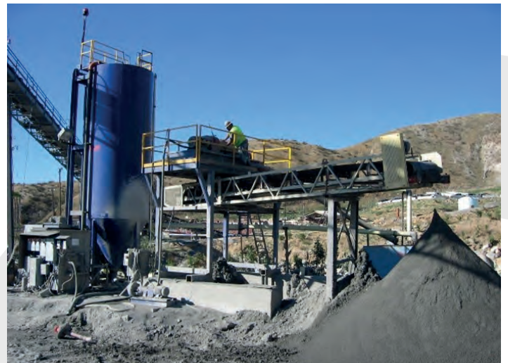
Figure 33: Arrowhead Tunnels – Spoil Treatment
