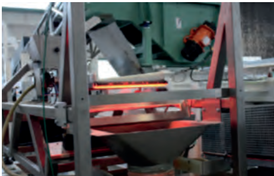
Figure 74: DRAGON Project – Instrumentation Photo-optical system to determine grain size and shape [[38]DP-4].
