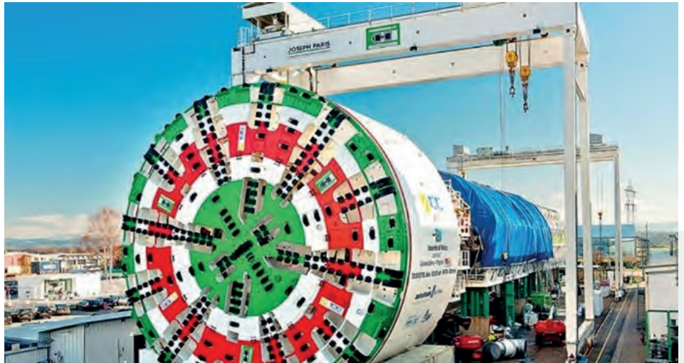
Figure 47: Sparvo Tunnel – EPB TBM at Plant General arrangement view of the EPB TBM at the Herrenknecht plant. (Courtesy of Herrenknecht AG)
