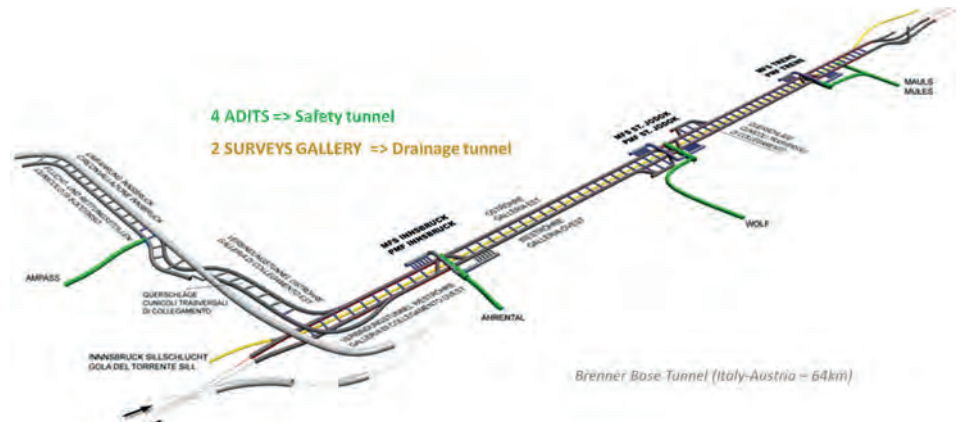
Figure 9 : Brenner tunnel, in green the 4 adits, in yellow a survey gallery all along the future base tunnel.
