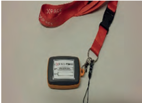
Figure 50 : Tunnel Tag required in order to allow the rescue team to localize the workers trapped in the tunnel.
