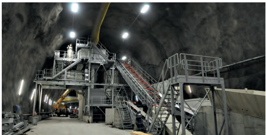
Figure 17 : Example of caverns for logistic installations (batching plant) in Ceneri.
