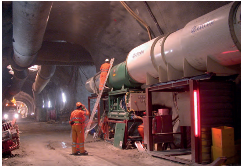
Figure 54 : Example of a mobile air cooling station for conventional drive on a sled.
