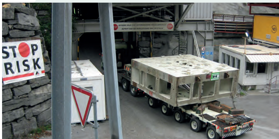
Figure 14 : GOTTHARD Tunnel, TBM Parts Transportation.
