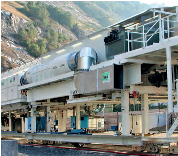
Figure 53 : Example of cooling equipment mounted on TBM.
