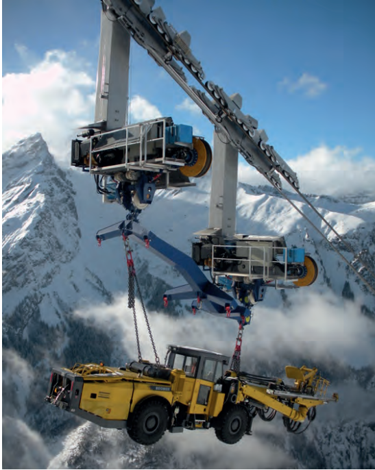
Figure 7 : Cable car for the Linthal Project, Switzerland, 2015 (Marti Tunnel Ltd).
