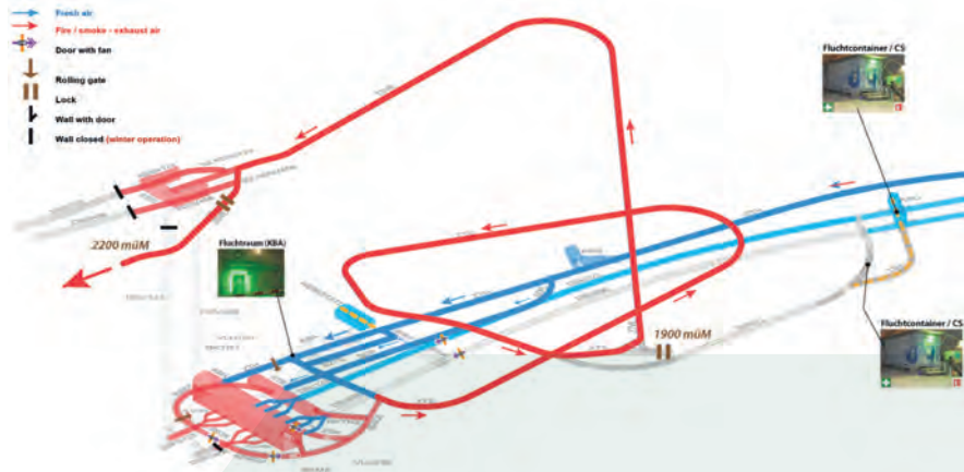
Figure 49 : Safety ventilation scheme – Nant de Drance 2015.
