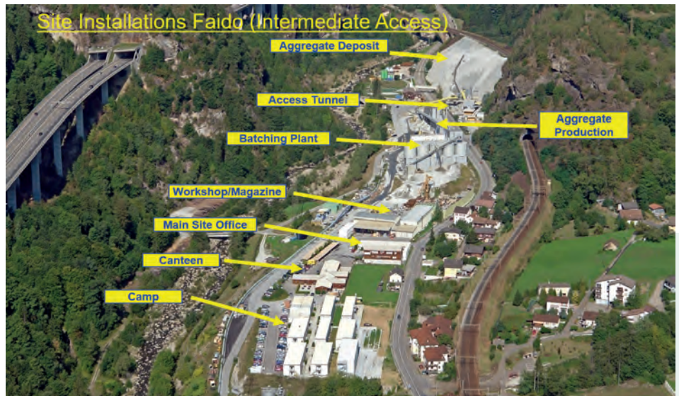
Figure 24 – Example for installations (conventional) in restricted space (Gotthard).
