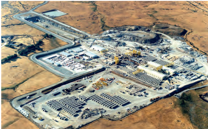
Figure 35 : Site set-up including space for temporary disposal of material in Guadarrama High Speed Rail Tunnels (courtesy ADIF).
