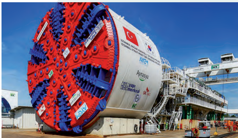
Figure 46: The Eurasia Tunnel TBM, designed for 13-bar hydrostatic pressure.
