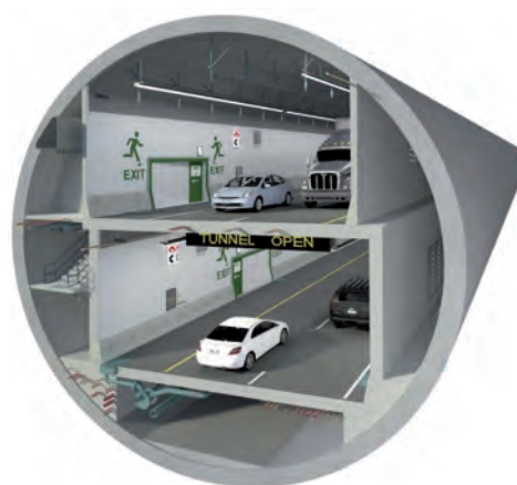
Figure 44: SR 99 bored tunnel cross section.
