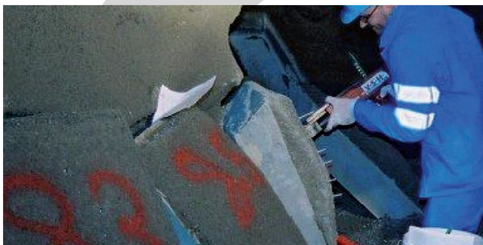
Photo 3: Measurement of early age strength of sprayed concrete.
