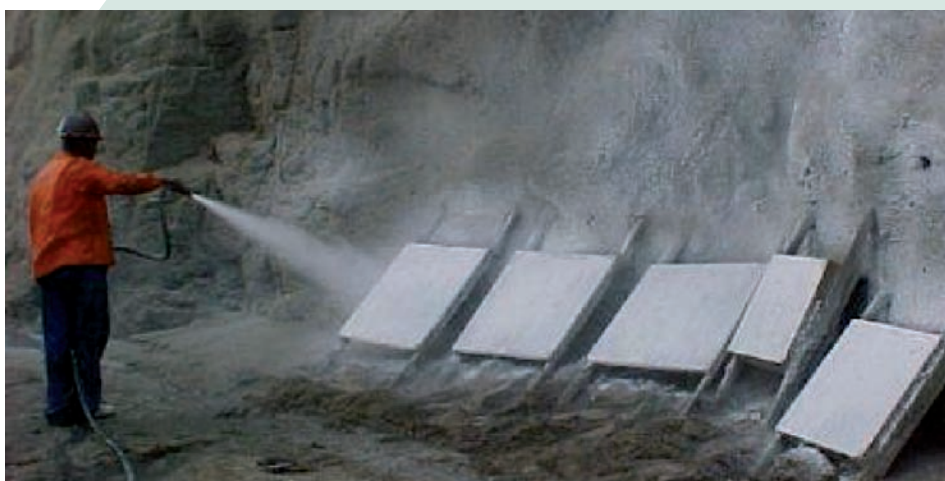
Photo 2: Tests for qualification of the sprayed concrete used in the tunnels.
