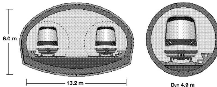
Fig. 7. Cross-section of bored tunnel showing cross-over (left) and running tunnel (right).
