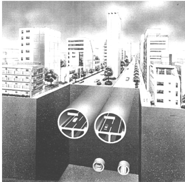
Figure 4-3 Typical tunnel structure of circular part
