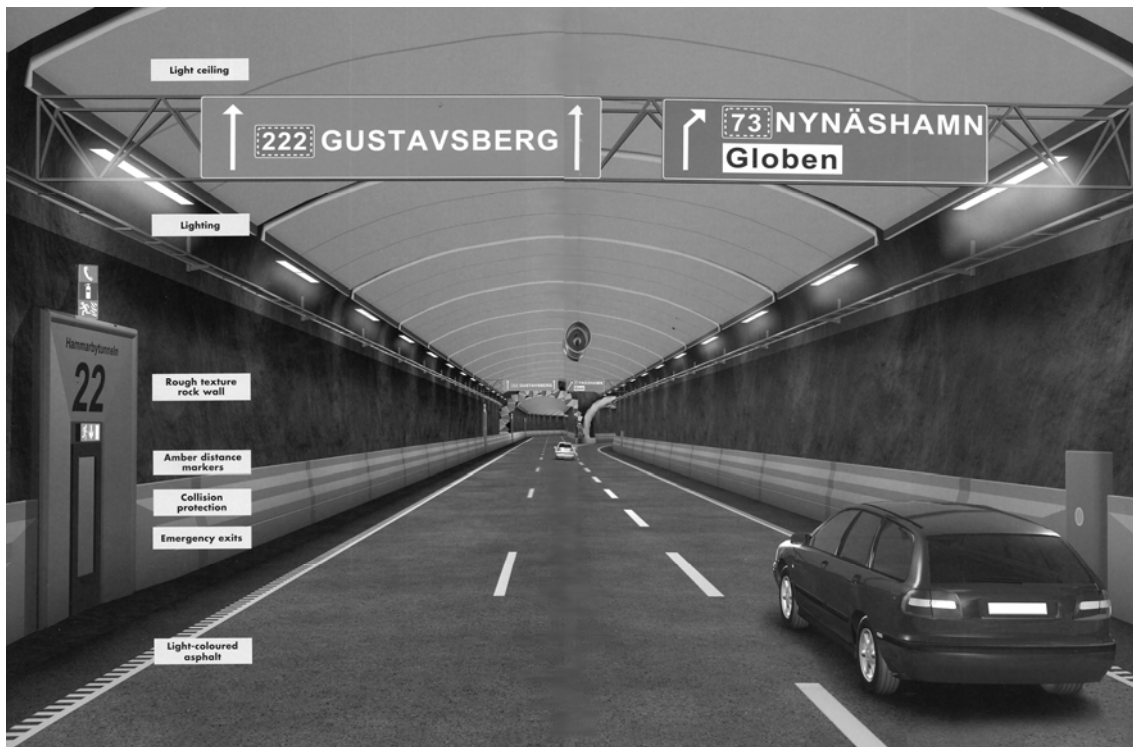
Interior of the Södra Länken road tunnel in Stockholm, Sweden (showing the light ceiling, the lightning, roch texture rock walls, amber distance markers, collision protection, emergency exits and the light-coloured asphalt) Total length of tunnel system including access tunnels 16.6 Km. Open for traffic October 24, 2004
