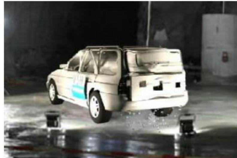
Blasting tests have been carried out with different charges to proof scalability of the model simulation.
