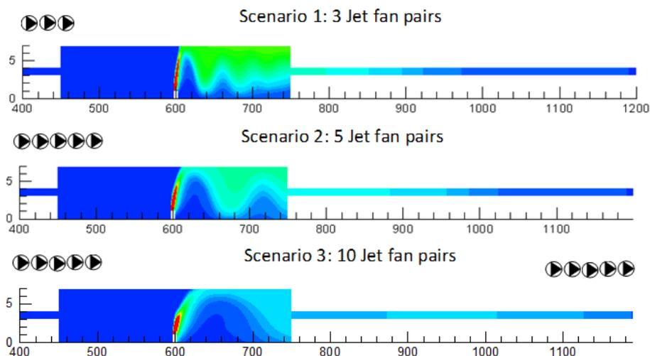
Figure 2. Example of time-dependent multiscale model results for a 30MW fire subject to different ventilation conditions.
