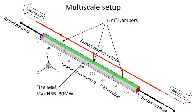
Figure 1. Example of multiscale model setup for the Frejus tunnel (Italy-France).
