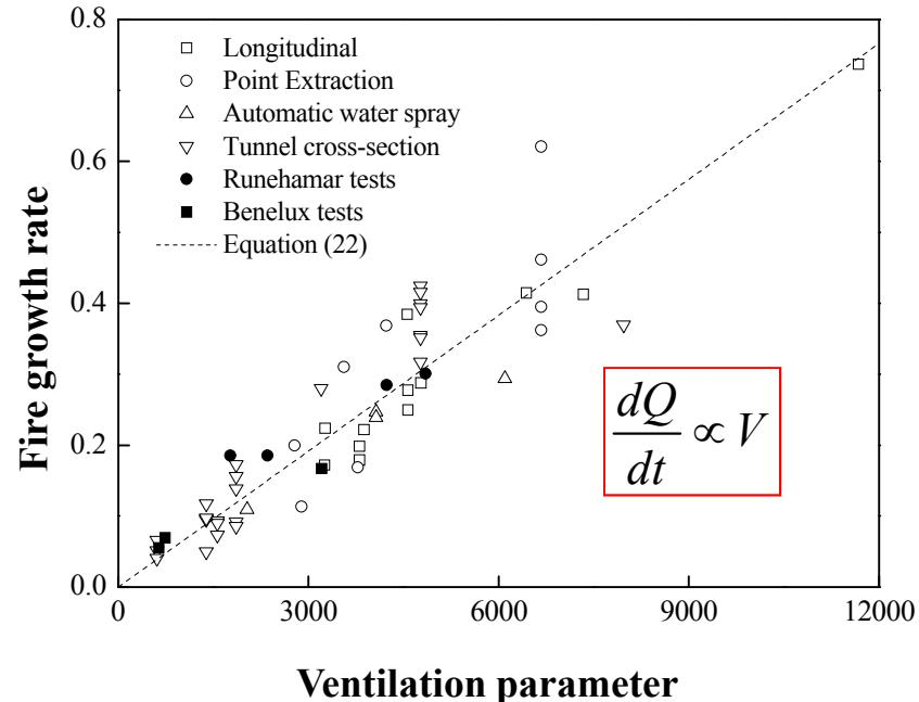
Fire growth rate **increases linearly** with ventilation velocity.
