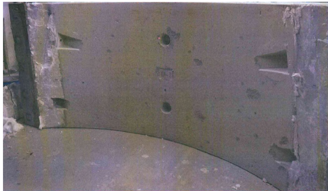
Pre-cast tunnel segment with PP fibre after fire testing
