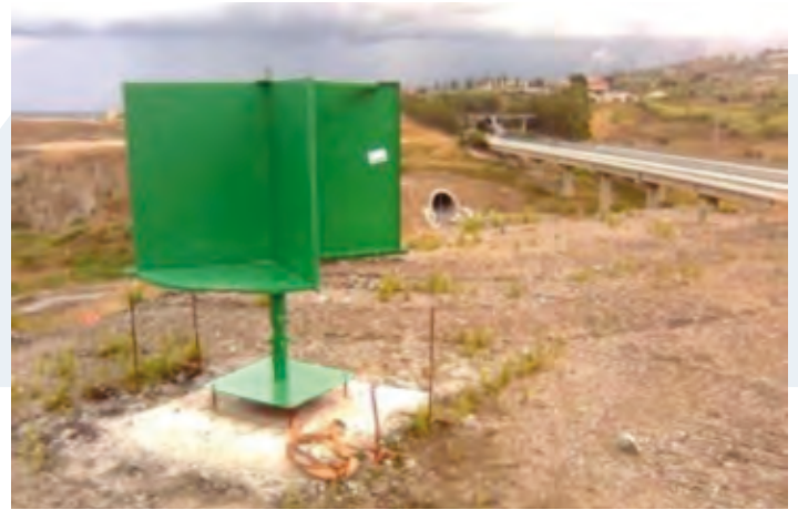
Figure 11. View of an artificial reflector installed on the slope of Tracoccia, Sicily; © Tele-Rilevamento Europa – T.R.E. Srl (TRE).
