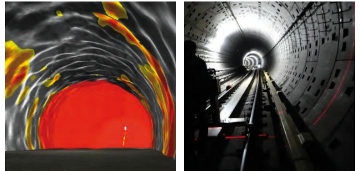
Figure 20 Deformation detection of SCL Linings (left) and deformation detection of inner lining segments (right).
