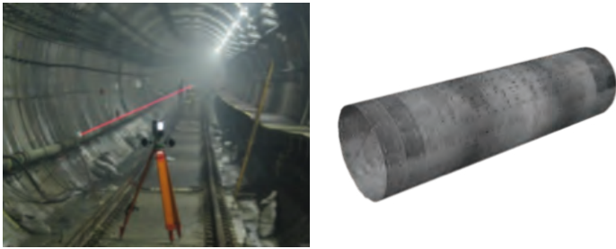
Figure 25 Stationary laser scanning in Beijing Metro Line (left) and the results in a 3D Viewer (right).
