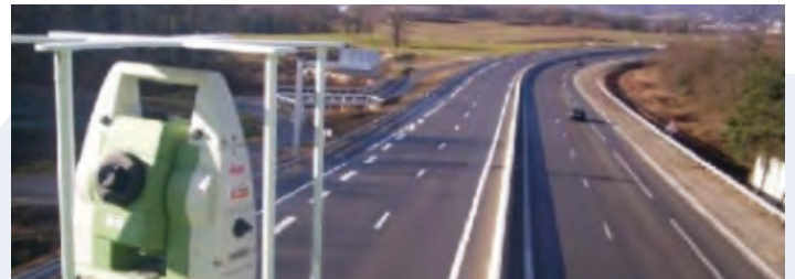
Figure 32 Reflectorless total station monitoring a motorway during construction of a service tunnel underneath.
