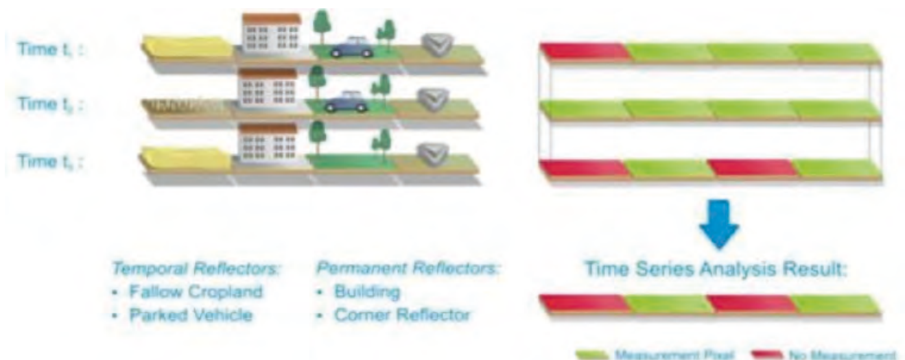
Figure 4. Types of Satellite Radar Interferometry reflector with surface movement information.
