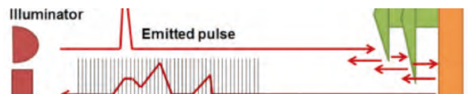
Figure 18. Full waveform digitization principle.
