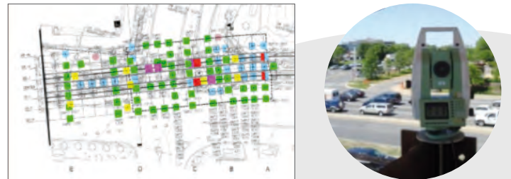
Figure 33 Total station on pillar with the monitored road (left), overview of monitoring points and their settlement values on road surface (right).
