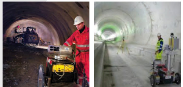
Figure 19. Stationary system on a trolley (left) and kinematic scanning system (right).
