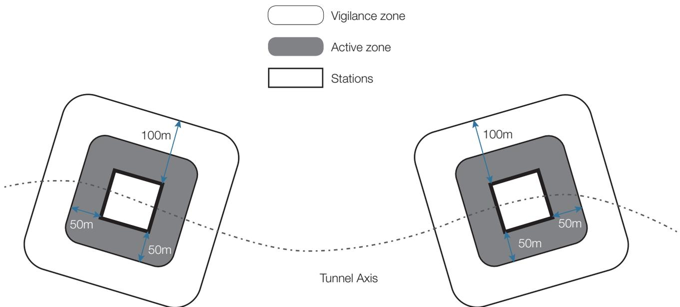
Illustration 2 : Diagram of the vigilance and the active zone, during the Station's construction
