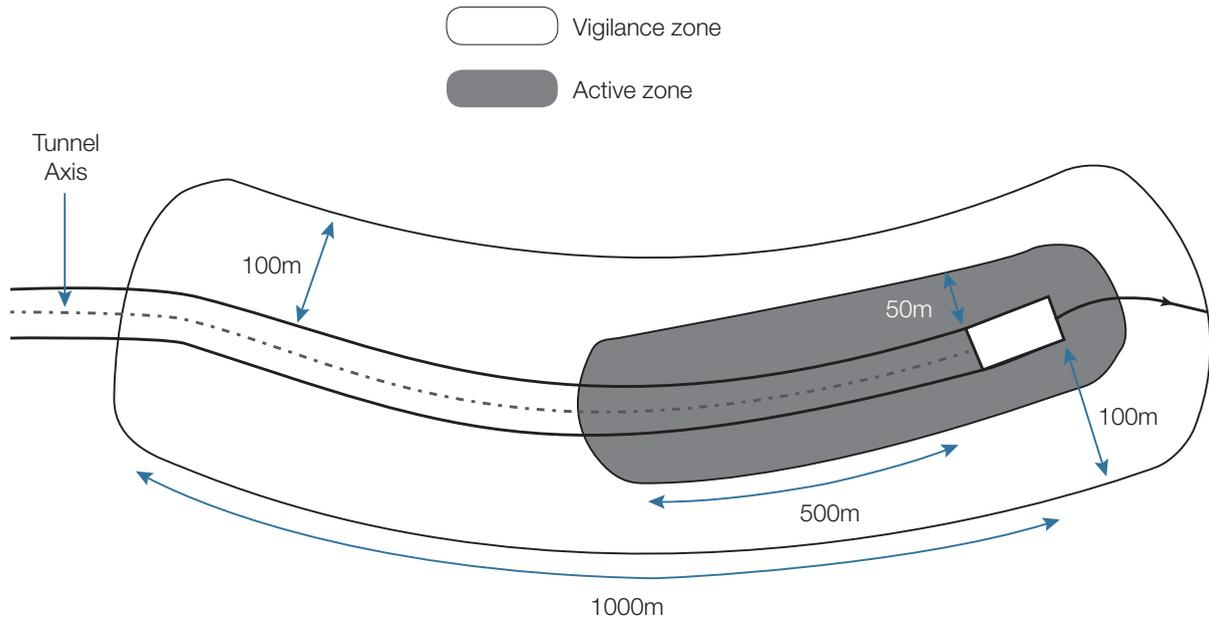
Illustration 1 : Diagram of the vigilance and active zones in running tunnel construction
