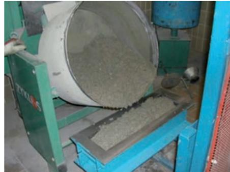
Figure 36 : Filling the mould of an EN14651 beam
