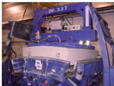
Figure 31 : Demoulding of key segment
