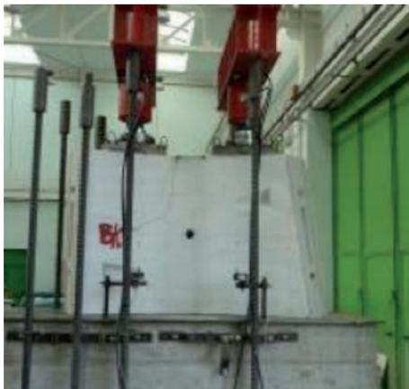
Figure 18 : Point load test set-up
