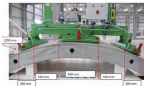
Figure 21 : Vacuum lifting system
