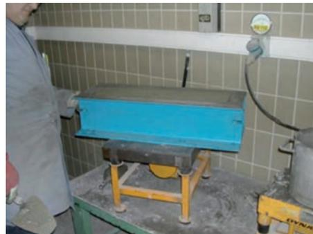
Figure 37 : Vibrating an EN14651 beam
