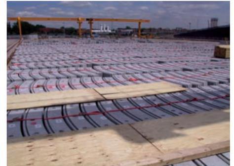
Figure 32 : Segments stacked at the factory
