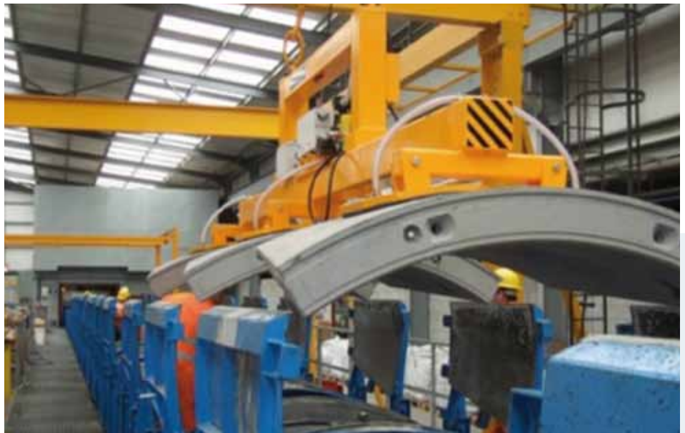
Figure 10 : Vacuum demoulding device for SFRC segments.
