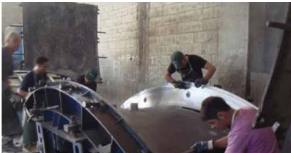
2 >> Cleaning of the mould.
