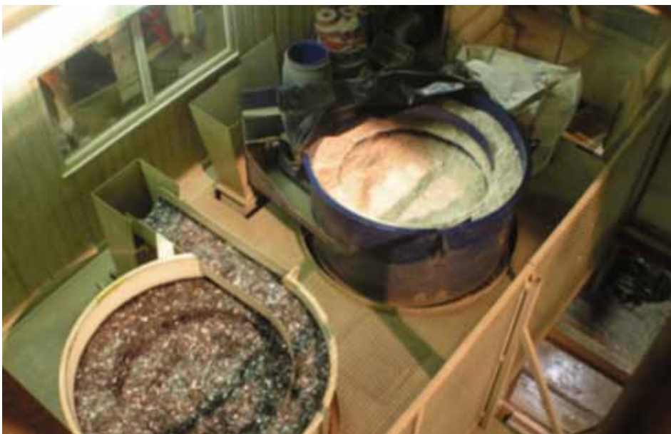
Figure 12 & 13 : Typical dosing equipment installed at the batching plant.
