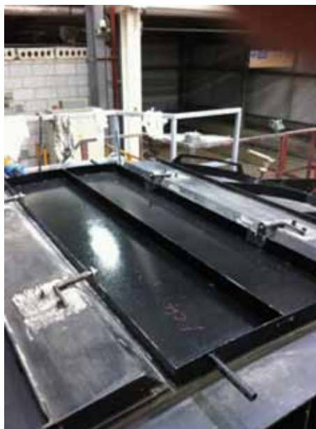
Figure 4 : Additional central extrados lid.
