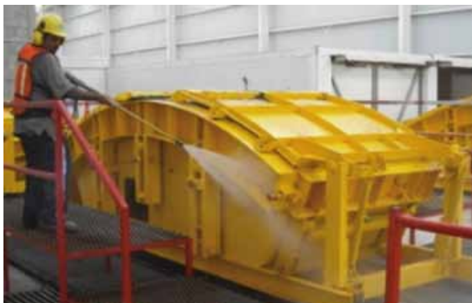
6 >> Cleaning the outside of the mould of residual concrete.
