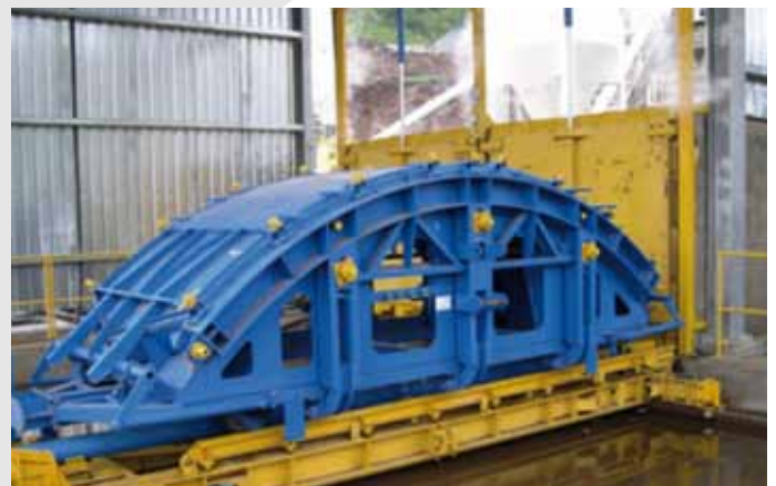
7 >> Preparing the mould for the curing tunnel.
