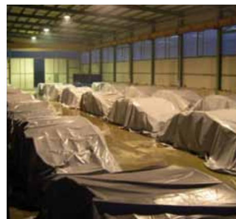
Figure 1c : Static moulds covered with thermal blankets.
