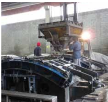
Figure 1b : Overhead bucket concrete delivery for static mould system.
