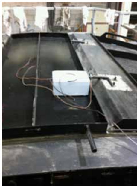
Figure 14 : Thermocouple based maturity monitoring system.
