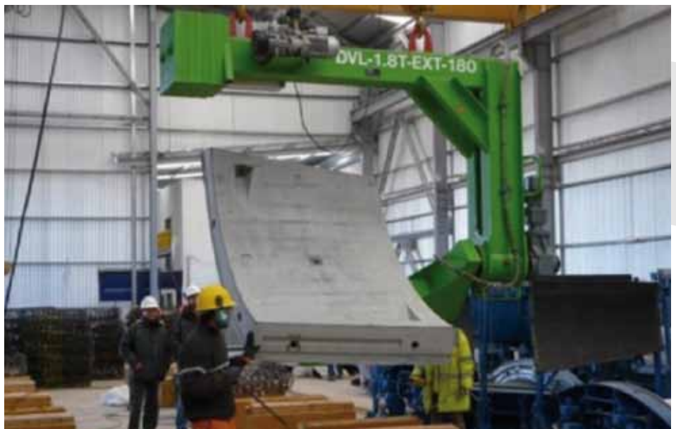
Figure 11 : Segment turning device.
