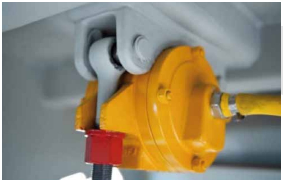
Figure 7 : Air vibrator beneath the mould intrados plate.
