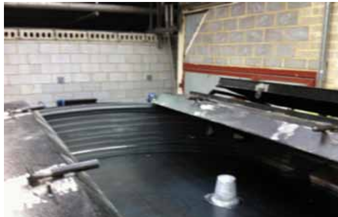
3 >> Preparing the mould for concreting. b. Placement of reinforcement cages, if required (not shown) and closing of the mould.
