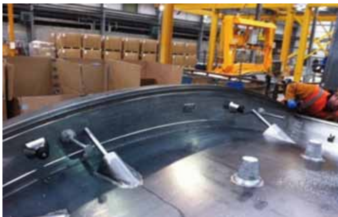
3 >> Preparing the mould for concreting. a. Placement of inserts, application of debonding agent, and greasing of the mould.
