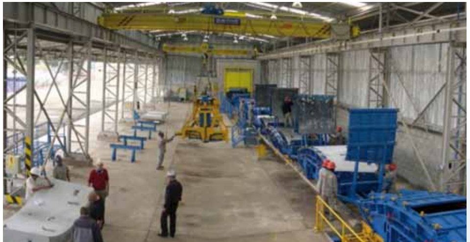
Figure 2 : A typical carousel system.
