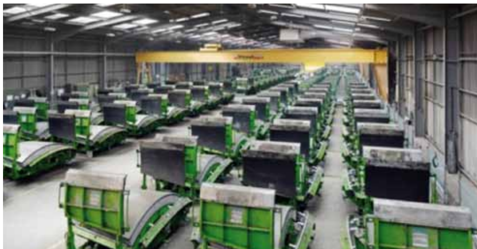
Figure 1 : Static mould system in a segment factory.
