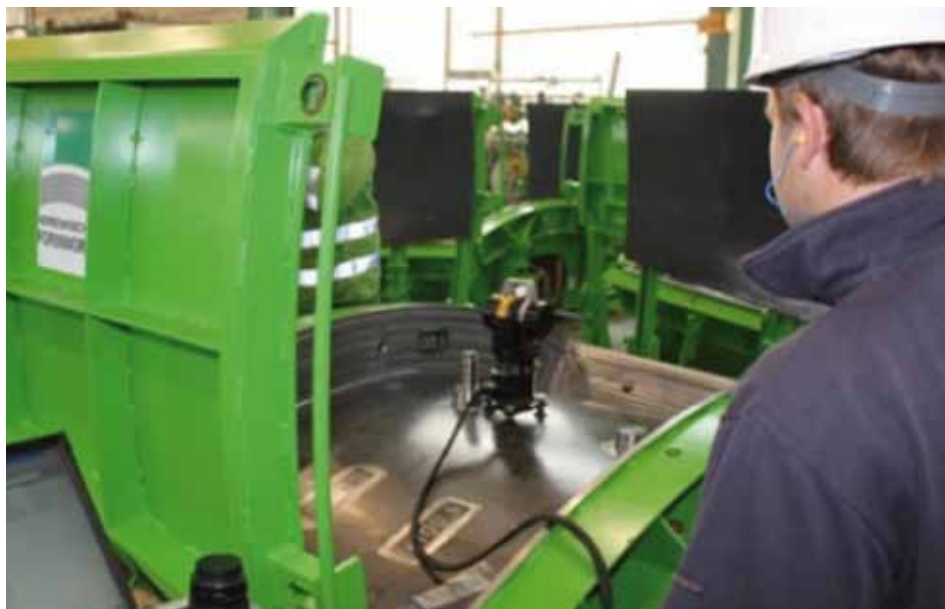
Figure 9 : 3D laser tracker checking of moulds.
