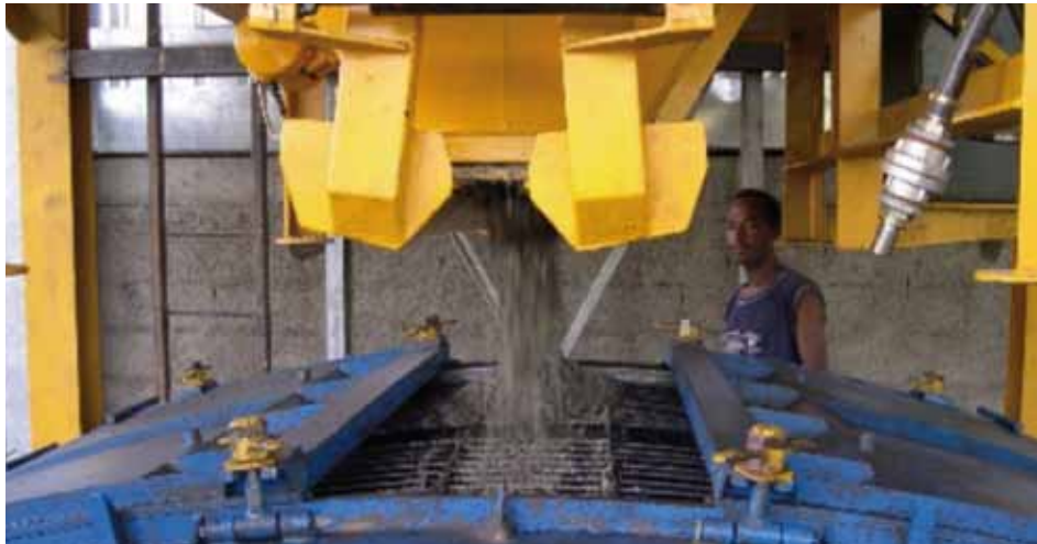
4 >> Placement of fibre reinforced concrete at the casting station.
