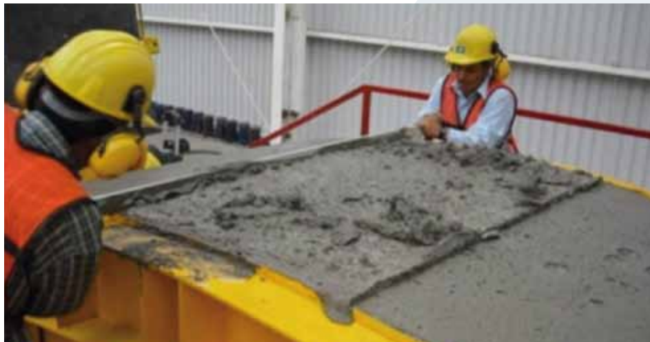
5 >> Trowelling of the segment extrados surface to remove entrapped air, if required, and closing of the mould lids before the mould is transferred into the heated curing tunnel.
