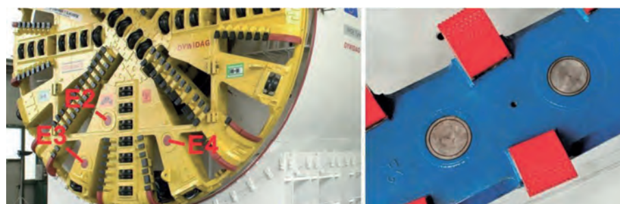
Figure 16 : SSP sensors, embedded into the cutting wheel, are continuously transmitting and recording data during advance [Herrenknecht AG].
