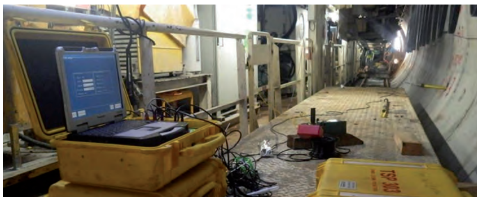
Figure 23 : TSP measurement in a mechanized tunnelling environment of a double shield TBM. Here, receivers and shot holes are set out thru the pre-cast segment lining.
