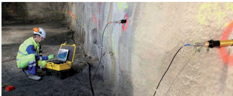
Figure 22 : TSP measurement in a conventional tunnelling environment. Here, two receivers and 24 shot points along the right tunnel wall side are shown.
