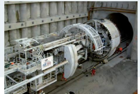
Figure 4 : Gripper TBM after refurbishment ready to be used for the Erstfeld contract of the Gotthard tunnel after completing the Amsteg section of the Gotthard tunnel
