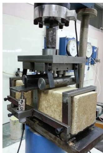
Figure 11: Four point bending test set-up
