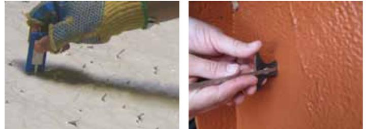
**Figure 6: Thickness control: wet film thickness testing**
