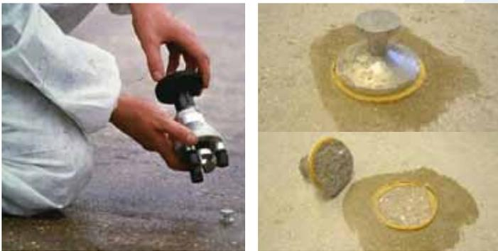
**Figure 9: Tensile bond test of horizontal substrate with elcometer. Dolly before and after testing (on the right)**
