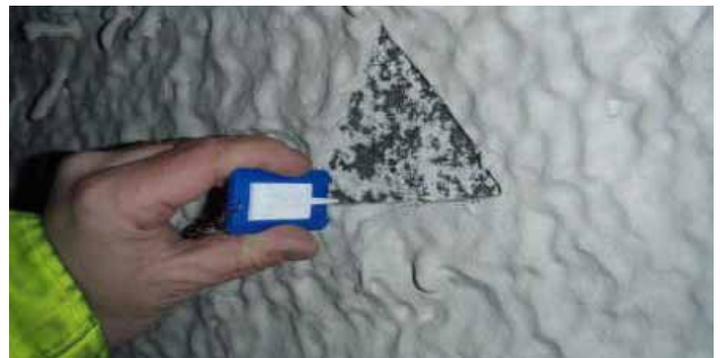
**Figure 8: Optional method with cut-out inspection patches to establish the applied membrane thickness**
