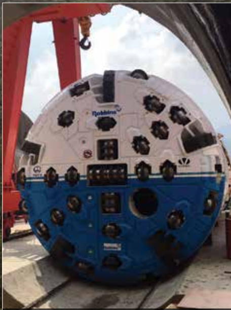
The 5.06m diameter Robbins Double Shield
